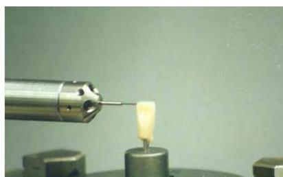
Fig. 4. The original tooth while measuring with Coordinate Measuring Machine (CMM)
