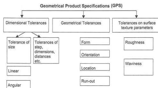
Fig. 5 General concept of “Geometrical Product Specifications” [6]
