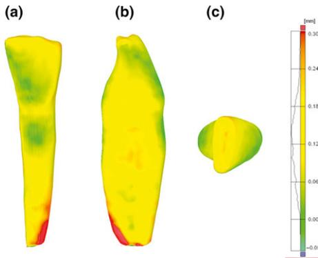
Fig. 2. Superimposed surfaces of the optical scans of the DLP 3D printed RAI and the original tooth. Measurement in millimetres. Frontal (a), sagittal (b) and occlusal (c) views. Notice: optical scan of the tooth served as the reference surface.
