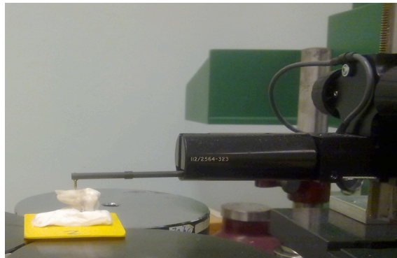
Fig.3. Schematic diagram illustrating Form Talysurf Intra 50 profilograph during the contact measurement of dental sample used in this study
